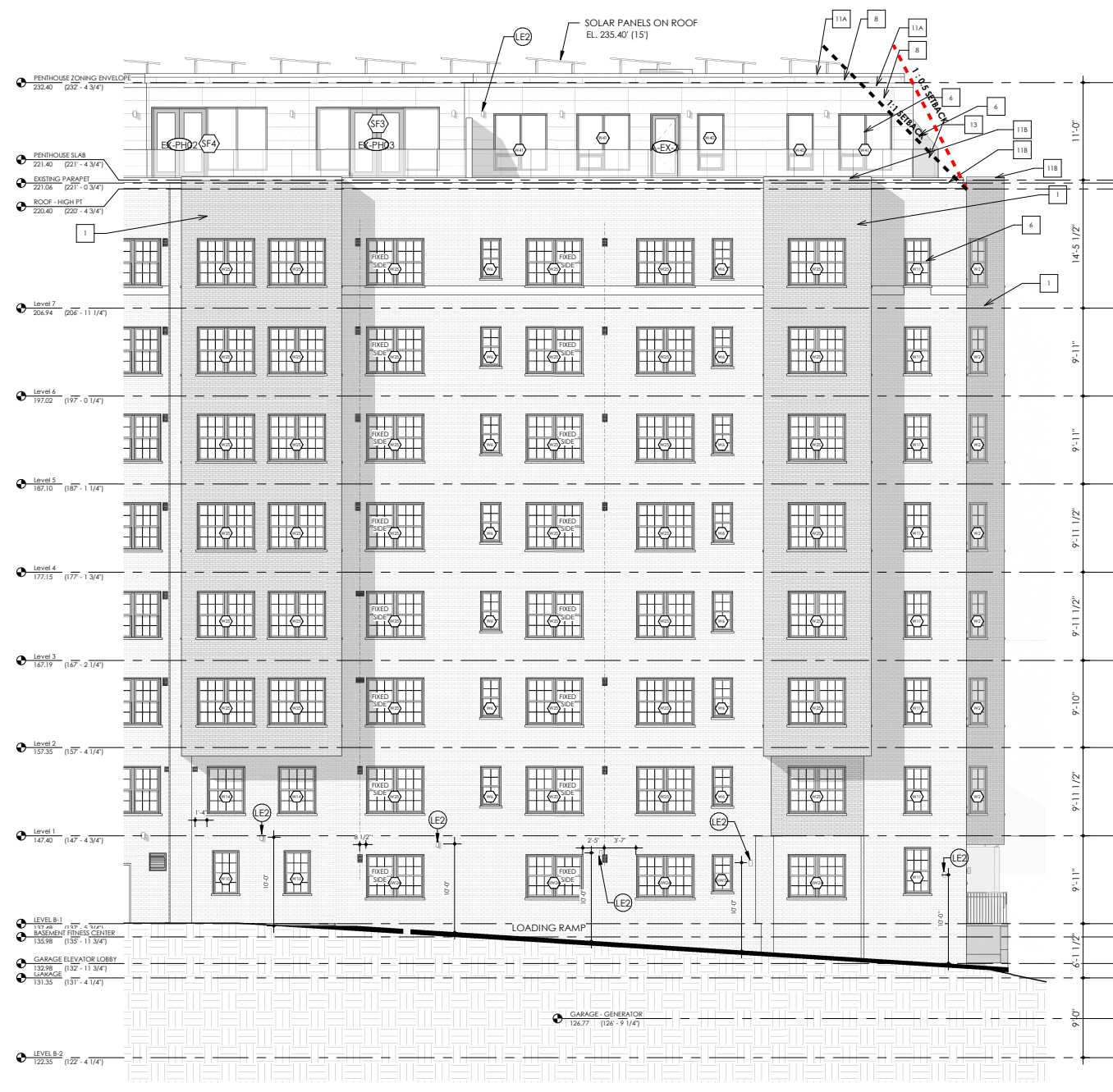
B5 PROPOSED - WEST ELEVATION - LOADING RAMP 1/8" = 1'-0"
